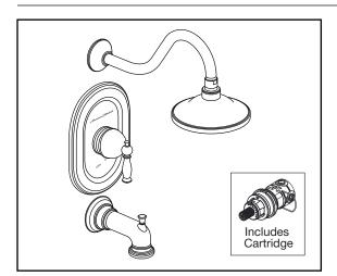
Pressure Balance Bath/Shower Trim with Double Ceramic Pressure Balance Cartridge
